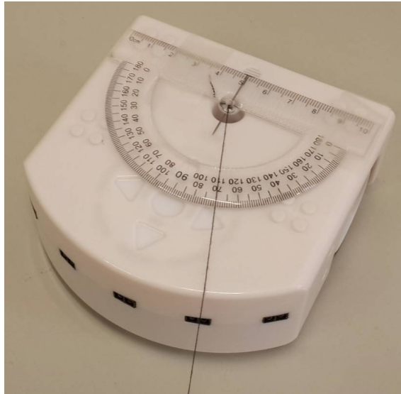
Figure 13.1: Measuring the angle between the sensors
